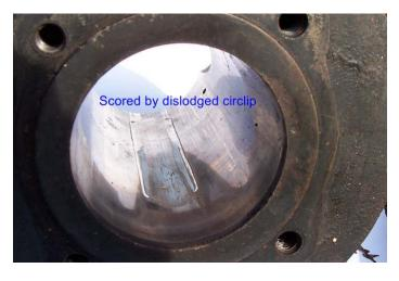
long enough to have created a superfluous two-stroke transfer port in the cylinder wall
