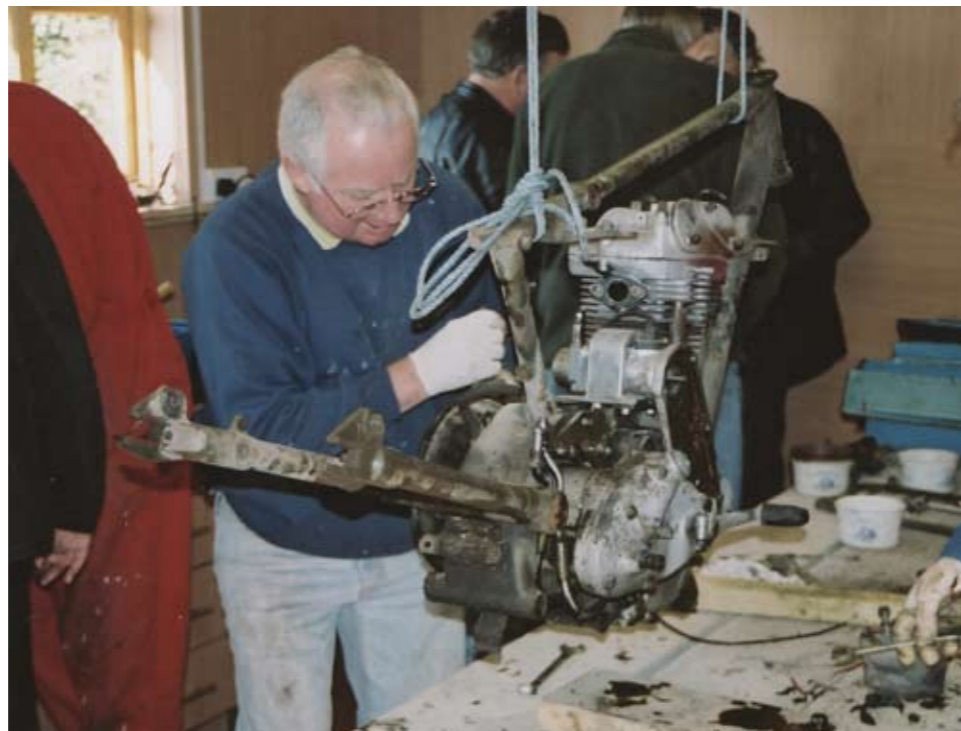
Main frame loop, engine and gearbox complete, and the swinging arm hanging from the rafters
